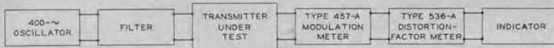
Layout for measuring distortion present in the output of a broadcast transmitter
