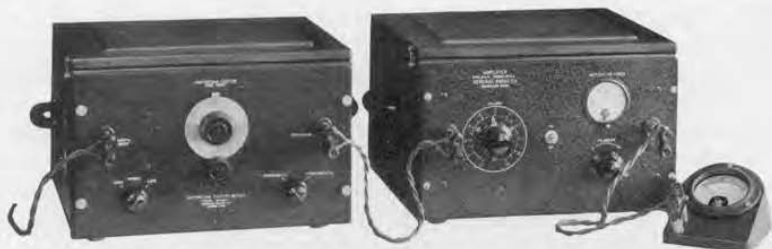
Apparatus for determining harmonic distortion. Left to right: TYPE 536-A Distortion-Factor Meter, TYPE 514-A Amplifier, and TYPE 488-HM Alternating-Current Galvanometer
