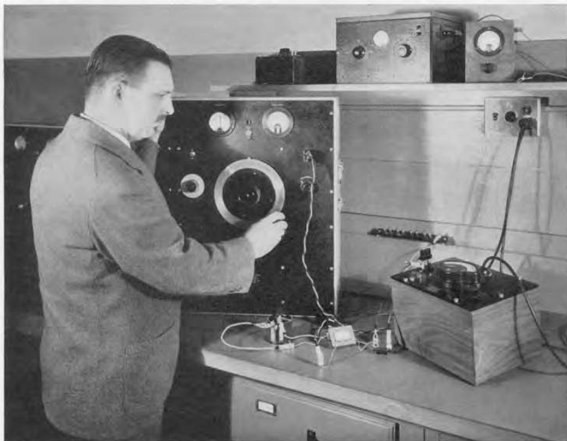
Measuring the response characteristic of an interstage coupling transformer with the TYPE 626-A Vacuum-Tube Voltmeter. The meter is on the bench at the right
